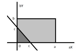
The area under the line equals to area of a right triangle with cathetus of length c:
