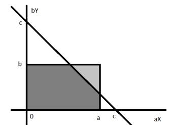
The area under the line equals to area of a right triangle with cathetus of length c minus area of a right triangle with cathetus of length (c-b) and minus area of a right triangle with cathetus of length (c-a):
