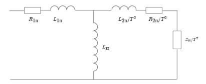
Where T – coefficient of voltage transform;  $L_{1n}$ ,  $L_{2n}$  – inductance of the primary and secondary windings associated with scattering;  $R_{1n}$ ,  $R_{2n}$  – active resistance of the primary and secondary windings, respectively.
