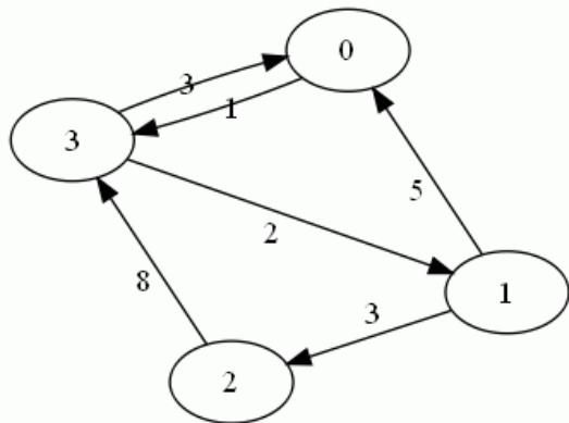
The figure above shows the directed weighted graph with 4 nodes and 6 edges. This graph can represent the railroad map where nodes are towns, edges are railroad routes between them, and weights are ticket costs in hundred dollars. For example, the fact that nodes 0 and 3 are connected by two directed edges with weights 1 and 3 means that the cost of travel from town 0 to town 3 equals to \$100, but the cost of travel from town 3 to town 0 equals to \$300.
