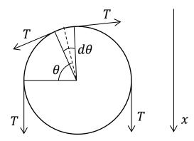
Let's consider a small angle  $d\theta$  as shown in the picture above. The normal to the cylinder surface at the middle of the segment (dashed line) bisects the angle  $d\theta$ . Thus projections on the normal of two forces T and T that act on this segment are the same and given by
