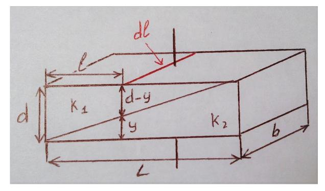
Hence, Plates' area of these smaller capacitors is  $b \cdot dl$ . Aggregate capacity of these two capacitors is
