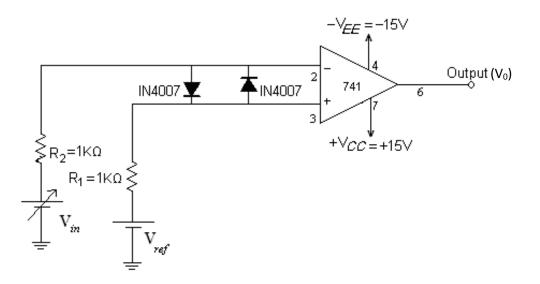
Design: A fixed reference voltage  $V_{ref}$  and varying voltage  $V_{in}$  is applied as shown in Fig. Vary the input voltage above and below the  $V_{ref}$  and note down the output at pin 6 ( $V_0$ ) of 741 IC.
