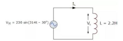
If the source were DC the inductor would just melt due to the high current passing through it as  $V_L$ = 0 in steady state. That is why one never connects and inductor across any DC source without resistance to limit the current in steady state. With AC this is not as problematic.
