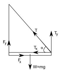
a) The sum of torques about the hinge must be equal to zero:
