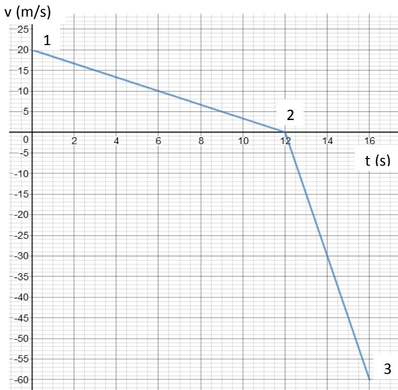
At initial time,  $t = 0$  s, the velocity is  $v = 20$  m/s. Put the point 1 on the graph that corresponds to these values. In  $t = 12$  s the velocity is  $v = 0$  m/s. Put the point 2 on the graph that corresponds to these values. Since a car decelerates uniformly draw a line 1-2. The area between the line and the time axis on a velocity-time graph, between two times is the displacement change  $\Delta x$  during that time interval. We find that
