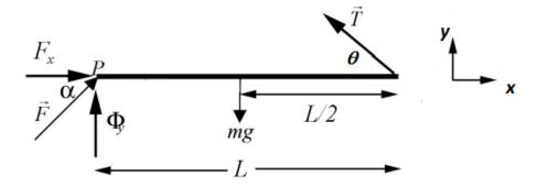
For static equilibrium, the sum of the forces must be zero, and hence the sums of the components of the forces must be zero;
