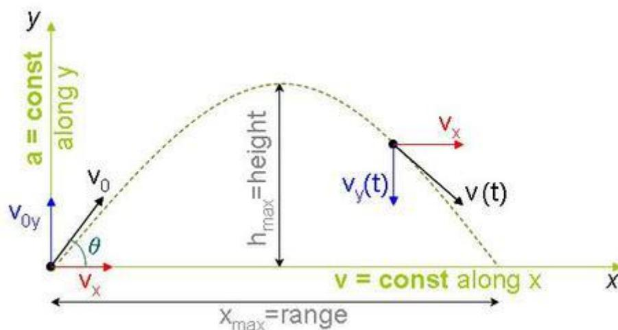
Projectile motion is a form of motion in which an object or particle (called a projectile) is thrown near the earth's surface, and it moves along a curved path under the action of gravity only.
