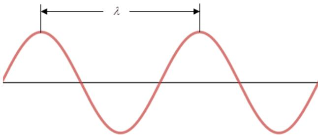
The wavelength corresponds to the distance that a point with a constant phase "passes" over a time interval equal to the period  $T$ , therefore we can find wavelength by
