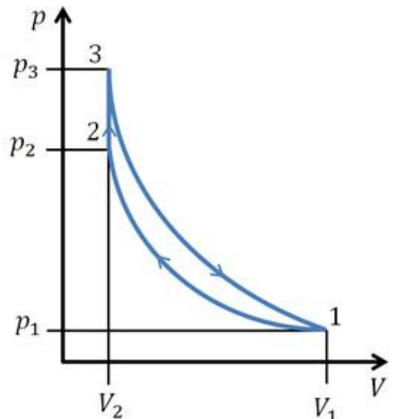
$$p_1 V_1^n = p_2 V_2^n. \quad (1)$$
