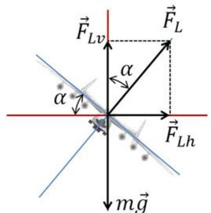
With the wings banked (see figure), the horizontal component of the lift is
