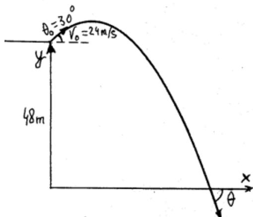
Treat the motion as two independent one-dimensional motions, one horizontal and the other vertical. The kinematic equations for horizontal and vertical motion of the spear take the following forms:
