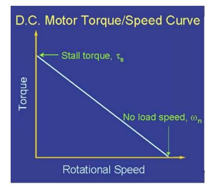
The graph above shows a torque/speed curve of a typical D.C. motor. Note that torque is inversely proportional to the speed of the output shaft. In other words, there is a tradeoff between how much torque a motor delivers, and how fast the output shaft spins. Motor characteristics are frequently given as two points on this graph:
