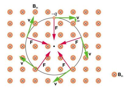
A negatively charged particle moves in the plane of the page in a region where the magnetic field is perpendicular into the page (represented by the small circles with x's—like the tails of arrows). The magnetic force is perpendicular to the velocity, and so velocity changes in direction but not magnitude.
