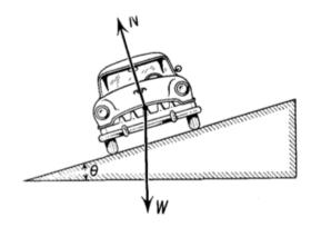
There are two forces acting on the vehicle: the weight, W (or mg), and the normal force, N. The y-component of the normal force neutralize the weight, and its x-component provides the necessary centripetal force for the curved motion of the vehicle, as shown in the force diagram below:
