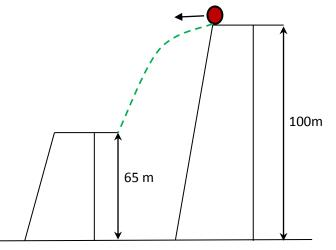
Consider the motion separately in horizontal and vertical direction (the trajectory shown in figure). In horizontal direction the body is moving uniformly with speed  $v_x = 70 \frac{m}{s}$ . In vertical direction the body is moving uniformly accelerated with acceleration  $g = 9.8 \frac{m}{s^2}$  downward. Therefore body height at an arbitrary time after the start of the fall, you can find as
