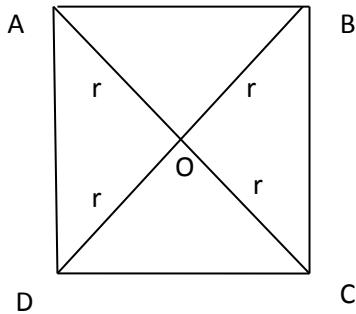
Force on the mass at the centre 'O' due to mass at A is:  $F_A = G \frac{m^2}{r^2}$  (1), where r is OA
