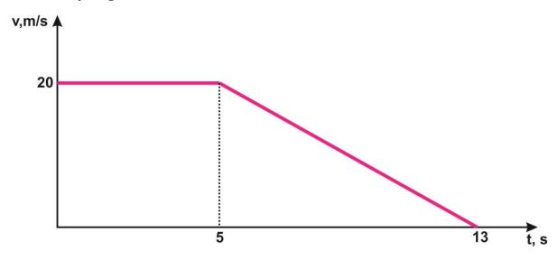
The area under the line in a velocity-time graph represents the distance travelled after the breaks are applied.
