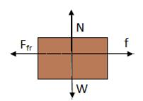
Write Newton's second law ma= f + W + N+ F<sub>fr</sub> ma =0 Ox: F<sub>fr</sub> = f Oy: N = W Friction force F<sub>fr</sub> =  $\mu$ N  $\mu$  W = f  $\mu$  = f / W  $\mu$  = 2.7 N / 7 N = 0.39 Answer: 0.39
