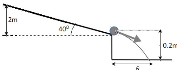
Find the speed with which a cylinder rolling on ramp
