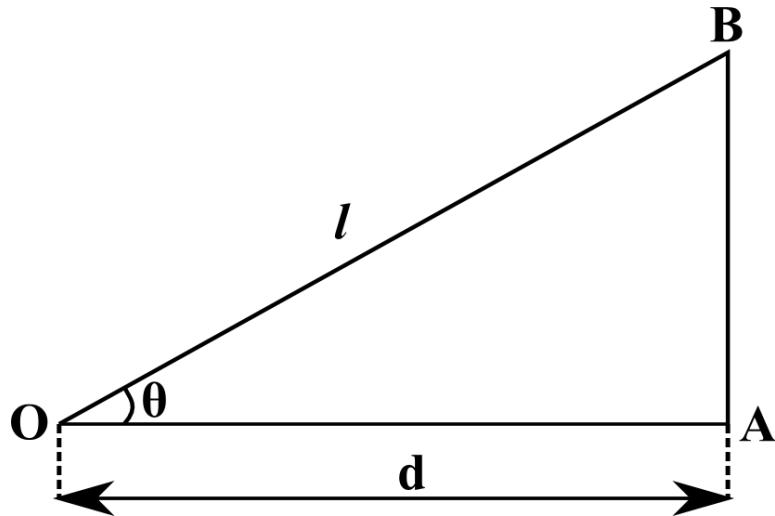
Let  $l = 7.85 \text{ m}$  is the length of the ladder,  $\theta = 66.5^\circ$  is the angle at which the ladder inclined to the horizontal and  $d$  is the horizontal distance from the bottom of the ladder to the building. Then, we can find  $d$  from the right triangle  $OAB$ :
