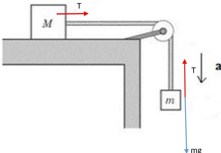
A frictionless pulley system is accelerated from rest. Using formula for path acceleration motion
