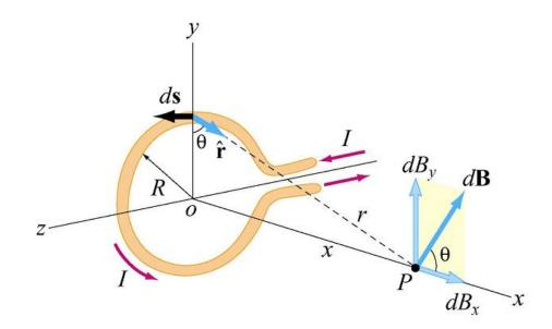
We have a 45 turn coil (here in the sketch depicted only one loop of the coil for simplicity) that has a radius of R = 0.183 m. The current that flows through that coil is equal to I = 2.81 A. Our task is to find the strength of the magnetic field at the point *P* on the coil's axis that is x = 0.483 meters from the center of the coil.
