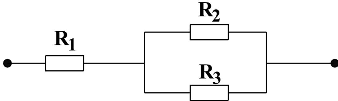
We have a  $R_1 = 1 \Omega$  resistor in series with a parallel arrangement of  $R_2 = 6 \Omega$  and  $R_3 = 3 \Omega$  resistors. Our task is to find the total resistance of the circuit.
