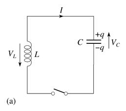
Let us consider some arbitrary time t after the switch is closed, so that the capacitor has a charge Q < Qmax and the current is I < Imax. At this time, both elements store energy, but the sum of the two energies must equal the total initial energy U stored in the fully charged capacitor at t=0:
