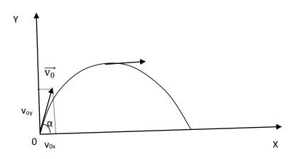
Elevation angle – the angle between of elevation line and of weapons' horizon line. From Figure  $\Rightarrow$  elevation angle  $\alpha=0^{\circ}$
