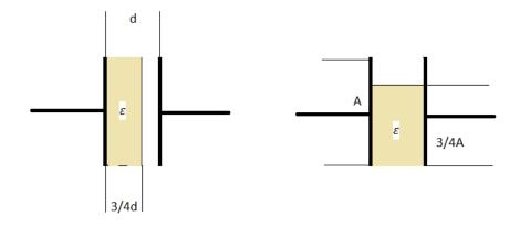
In the first case we can consider the capacitor to be series connection of two capacitors.
