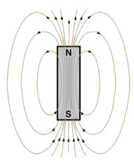
The lines of magnetic field from a bar magnet form closed lines. By convention, the field direction is taken to be outward from the North pole and in to the South pole of the magnet.
