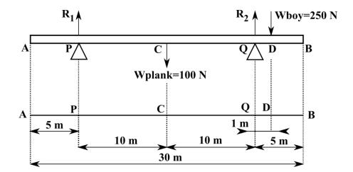
a) To find the reaction force at the left support,  $R_1$ , we should consider the sum of moments of forces around the point Q. From the condition of the question we know that the arrangement is in equilibrium, thus the sum of all moments is equal to zero:
