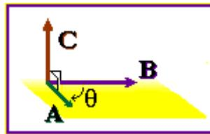
Moment of force (or torque) is example of the cross product of the lever-arm distance vector and the force vector, which tends to produce rotation:
