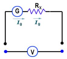
Let the resistance of galvanometer be  $R_g$  and high resistance  $R_x$  is connected in series to it. Then combined resistance will be  $(R_g + R_x)$ . Therefore, from the Ohm's law we can write the potential between the points to be measured:
