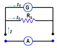
Let the resistance of galvanometer be  $R_g$  and it gives full scale deflection when current  $I_g$  is passed through it. Then, from the Ohm's law we can write the potential difference across the galvanometer:
