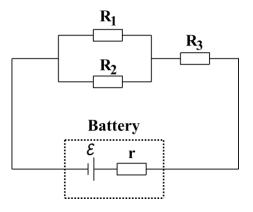
We have a parallel combination of  $R_1 = 2 \Omega$  and  $R_2 = 3 \Omega$  resistors that are connected in series to a  $R_3 = 4 \Omega$  resistor. The combination is then connected across a 12 V battery having internal resistance of  $r = 1 \Omega$ . Our task is to find the equivalent resistance of the circuit.
