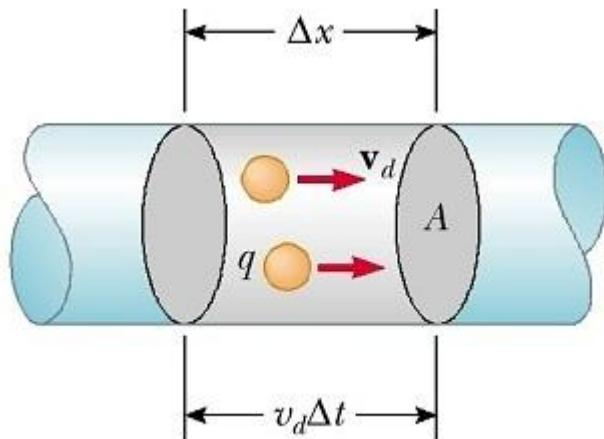
The volume of a section of the wire of length  $\Delta x$  (the gray region in the picture above) is  $A\Delta x$ . If  $n$  is the number of free electrons per unit volume, then the number of free electrons in the gray section is  $nA\Delta x$ . Then, we can write the charge  $\Delta Q$  in this section:
