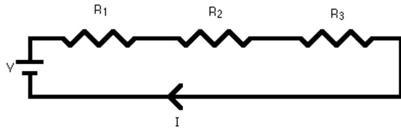
a) Let's first find the equivalent resistance of resistors in series:
