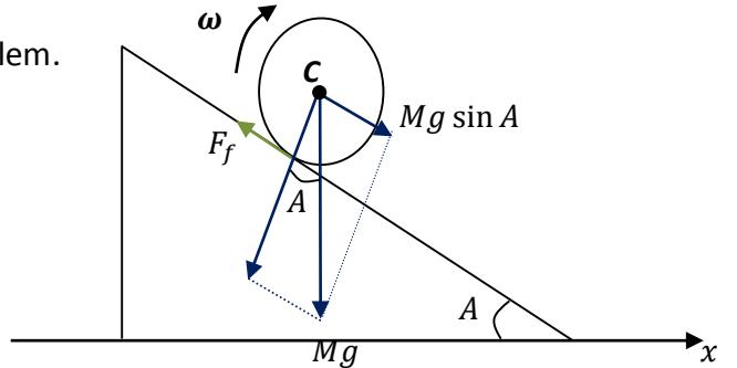
Projection of the force of gravity on an inclined plane is equal to  $Mg \sin A$ .
