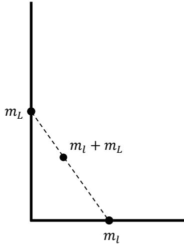
Let the length of the vertical section be  $L$  and mass  $m_L$ . Its center of mass lies at the center of it. The same is true for the horizontal section which's length is  $l$  and mass  $m_l$ . Distance between these two centers is
