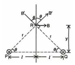
Situation of the problem is shown in the adjoining figure. Points Q and P represent two wires, each carrying current along inward normal to plane of the paper. It is given that each of these two wires carries a current *I* and separation between the wires is 2*l*. In the figure, dotted line PQ represents the plane of wires and solid line normal to PQ represents the plane of symmetry.
