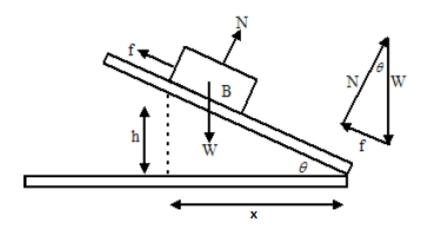
It is found experimentally that the force of friction f is proportional to the normal component N of the plane's reaction. Stated algebraically
