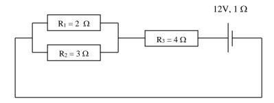
Since R1 and R2 are in parallel, their equivalent resistance is calculated:
