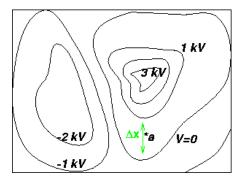
The figure shows equipotential lines. The electric field at point a can be found by calculating the slope at a:
