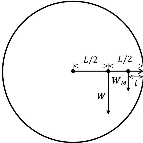
The forces which act on the Hour hand are shown in the figure above. Since the pull-ups is the periodic process the net force acting on the Hour hand due to Mario's weight is  $W_M$ . Therefore the net torque around the pin is given by
