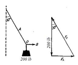
We know that the junction 0 is in equilibrium under the action of these forces, hence their resultant must be zero. Therefore, the vectors representing the three forces can be combined to form a closed triangle, as shown at the right in Fig.
