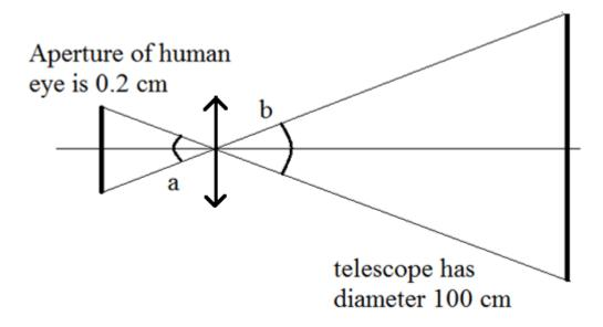
As the angle A equal to the angle B thus from the similarity of triangles we have the minimum magnifying power of a visual telescope 100/0.2=500.
