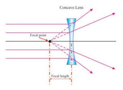
As we can see in the picture, concave lens are thinner at the middle. Rays of light that passes through this lens are spread out, so the concave lens is a negative or diverging lens.
