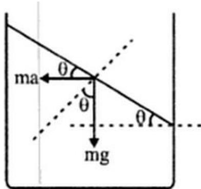
This is the position of the liquid surface with respect to frame of the tank.
