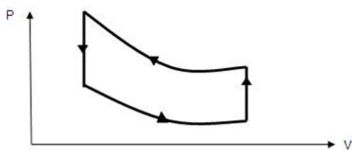
The counterclockwise thermodynamic cycle indicated by the arrows shows that the cycle represents a refrigerator. So, the work is done on the gas.
